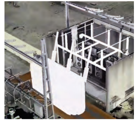
Sequencing animation that shows the temporary works coming in then the replacement unit.
